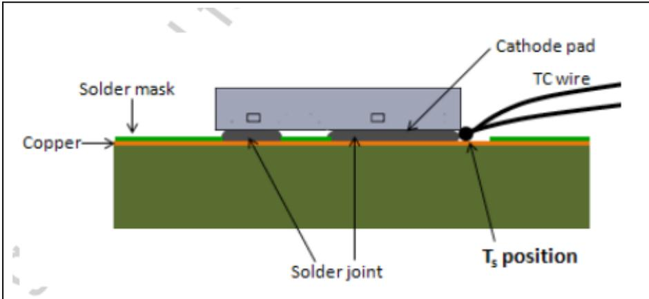
Thermocouple Location on Temperature Measurement Point (TMP):
