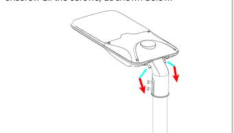
5. Rotate the lamp to a proper Angle (up to 12 degrees, down to 12 degrees) , then tighten the two bracket screws, as shown below.
