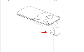
4. Unscrew the two screws of the bracket (do not unscrew all the screws) as shown below.
