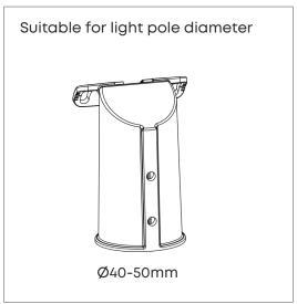
If the fixture is installed by post top, please release the screws on the bracket behind the fixture and remove the bracket first, then turn the bracket in the opposite direction, use wrench to tighten the screws to fix the bracket, as shown below.
