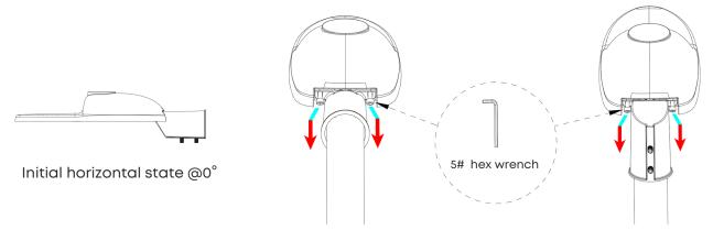
5. Rotate the fixture to the proper angle based on the actual requirement, then tighten two screws behind the fixture on the bracket.
