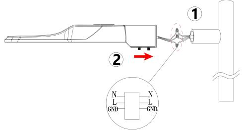
Diagram of correct and incorrect fixation of lamp pole and bracket.
