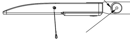
Torque force  $\geq 8.5\text{N}\cdot\text{m}$  until locking
