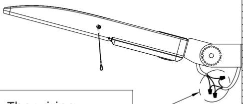
Note: The wiring terminals are waterproofed with glue or connected with waterproof connectors.
