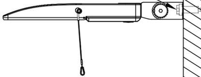
Step 3 - Fix the fixture on the wall or ceiling
