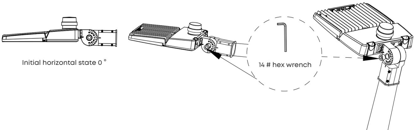
5. Rotate the lamp to the appropriate angle according to actual needs, and then tighten the fixing screws on the bracket
