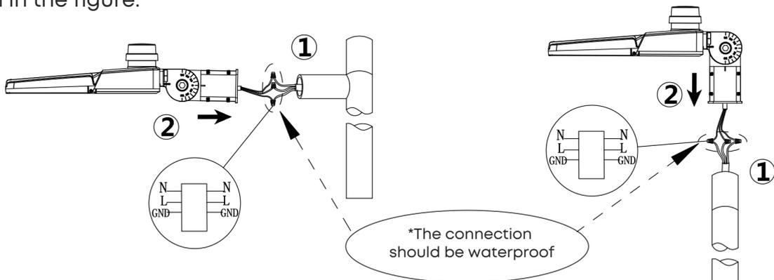
Installation and fixing diagram of lamp post and bracket
