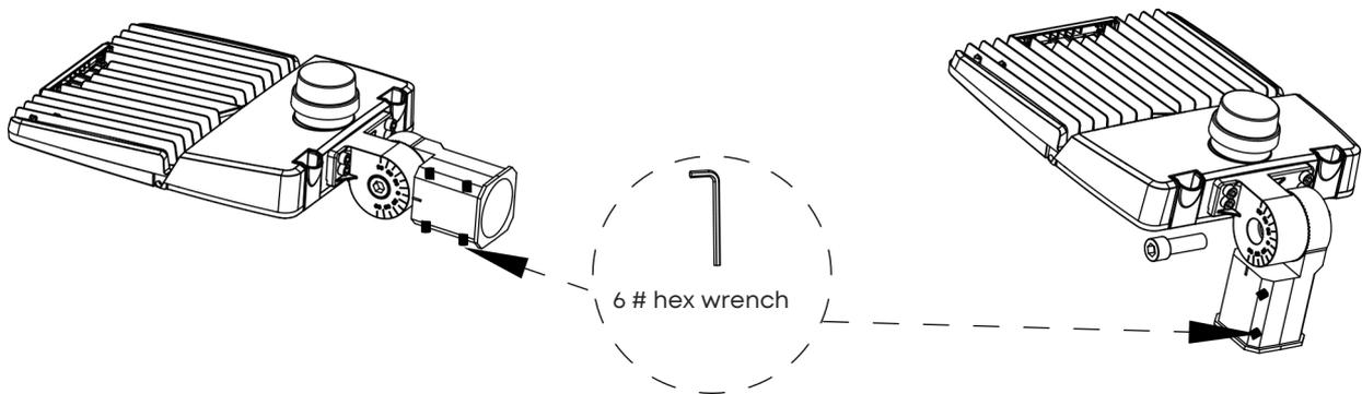
2. Connect the wires between the lamp bracket and the lamp post (connect L, N, GND respectively), and then insert the bracket into the lamp post in the direction of the arrow as shown in the figure.
