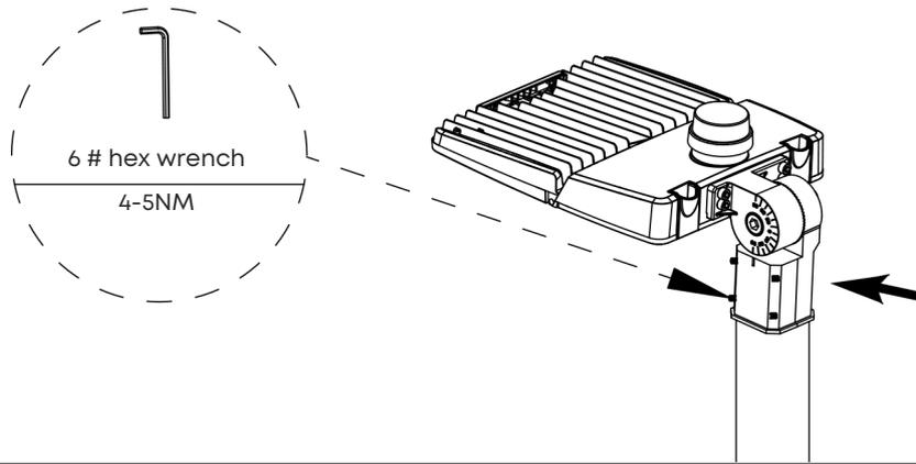
4. If angle adjustment is required, loosen the screw 2-3 turns and do not completely unscrew the screw
