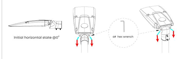
5. Rotate the fixture to the proper angle based on the actual requirement, then tighten two screws behind the fixture on the bracket.
