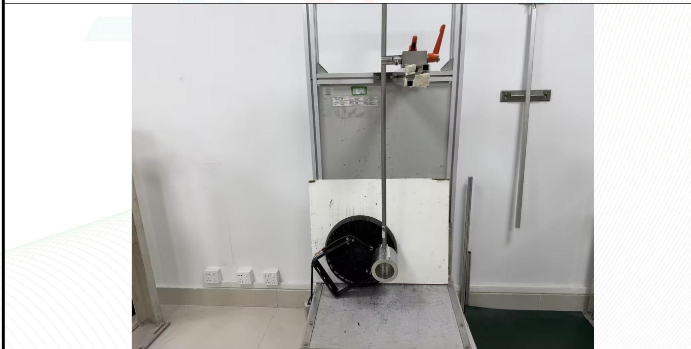
Photo 4: IK10 test of model AOK-200WHBE-NV-L2-00-6570-60-P
