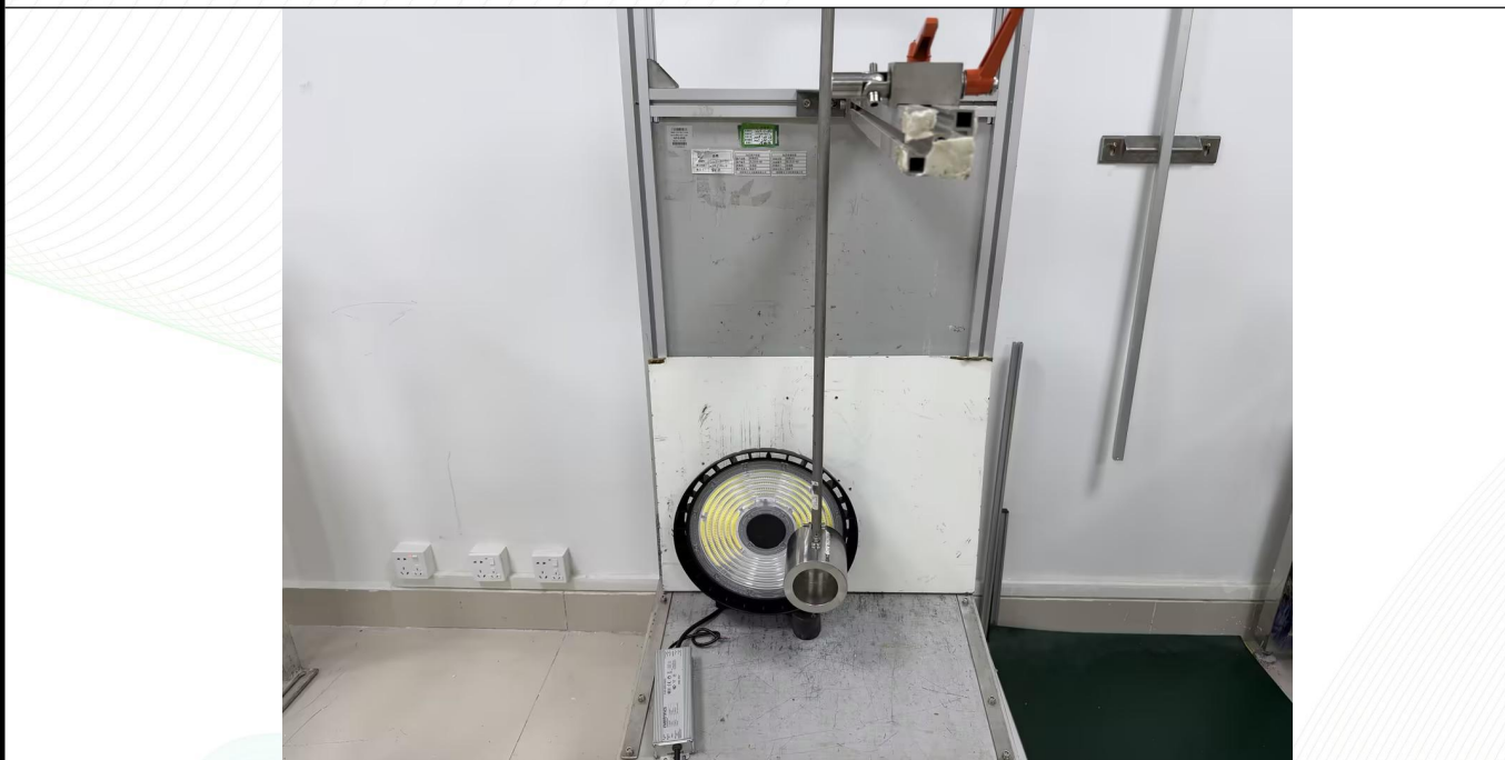
Photo 3: IK10 test of model AOK-200WHBE-NV-L2-00-6570-60-P
