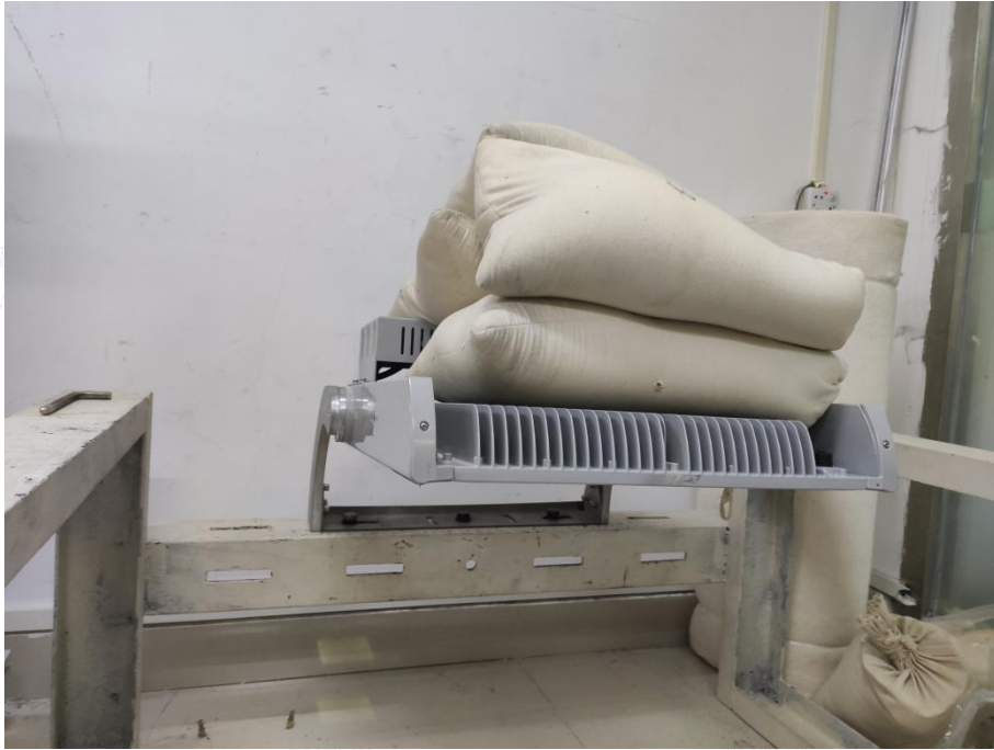
Photo 3: Test result of Static Load Test
