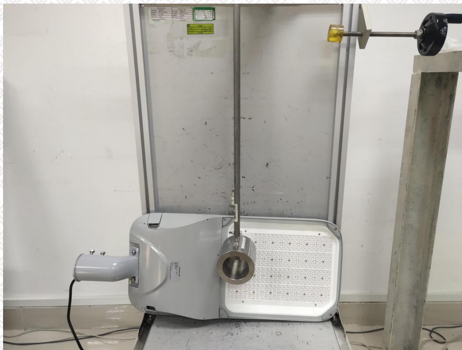
Photo 3: IK08 test of model AOK-200WiL02-NV-L3-00-40
