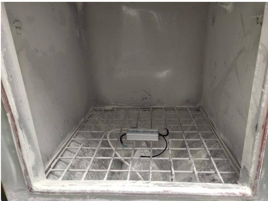
Photos 2: IP6X test of model EUM-200S560MG
