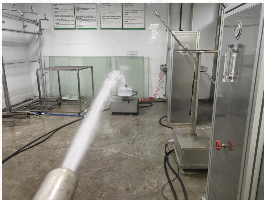
Photo 4: IPX6 test of model AOK-200WiL02-NV-L3-00-40
