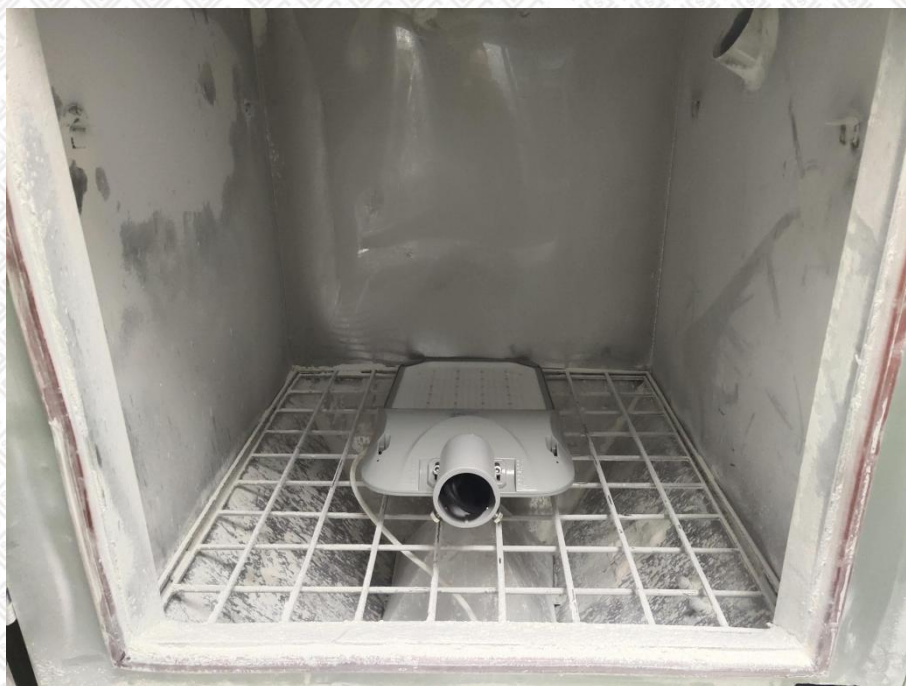
Photo 3: IP6X test of model AOK-200WiL02-NV-L3-00-40
