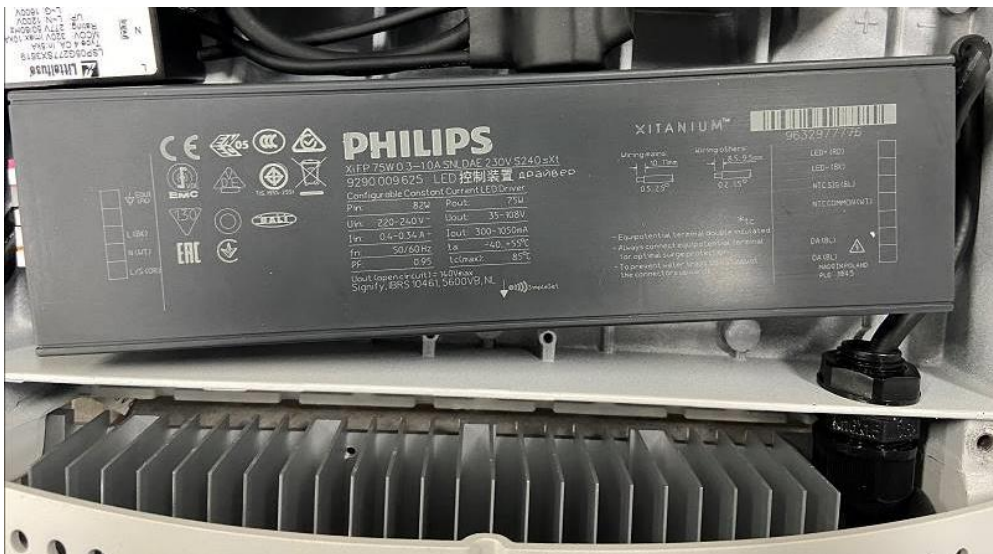
Picture 4: LED driver view [Model: Xi FP 75W 0.3-1.0A SNLDAE 230V S240 sXt]
