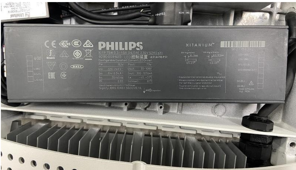
Picture 4: LED driver view [[Model: Xi FP 75W 0.3-1.0A SNLDAE 230V S240 sXt]
