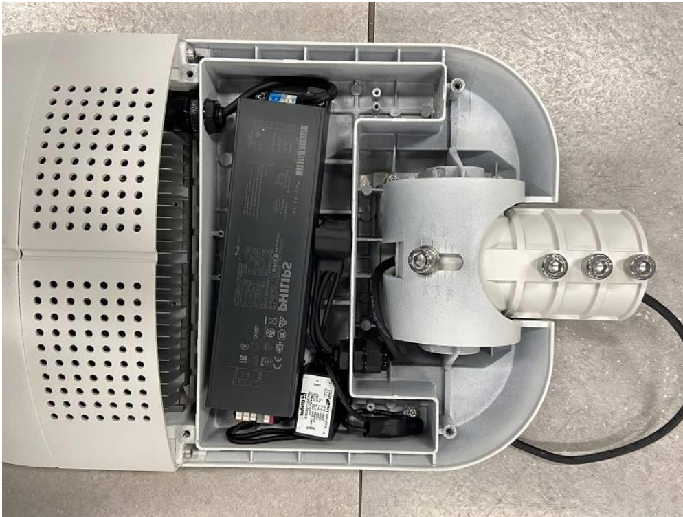
Picture 4: LED driver view [Model: Xi FP 75W 0.3-1.0A SNLDAE 230V S240 sXt]
