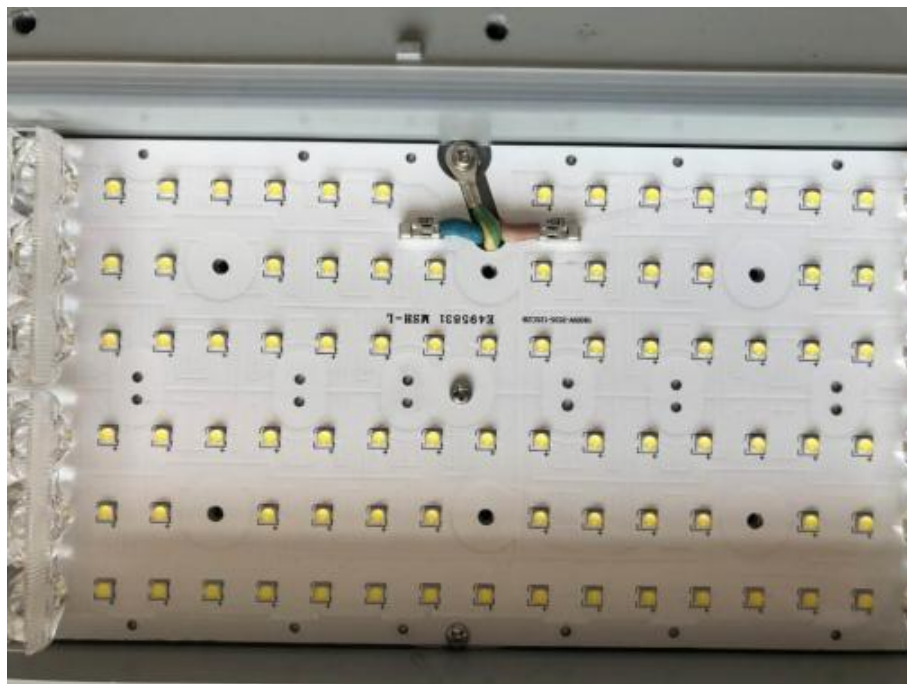
Figure 4 LED (3535) module view of model AOK-1800WiSF-HV-DV-S35-6570-15-U
