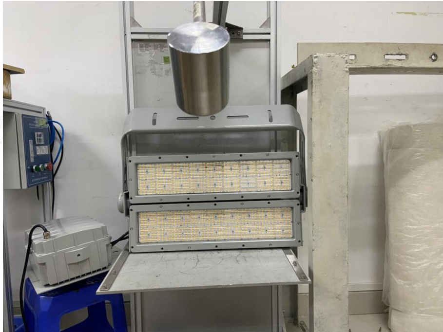
Photo 3: IK08 test of model AOK-1200WiSF-HV-00-S5-5070-30-U
