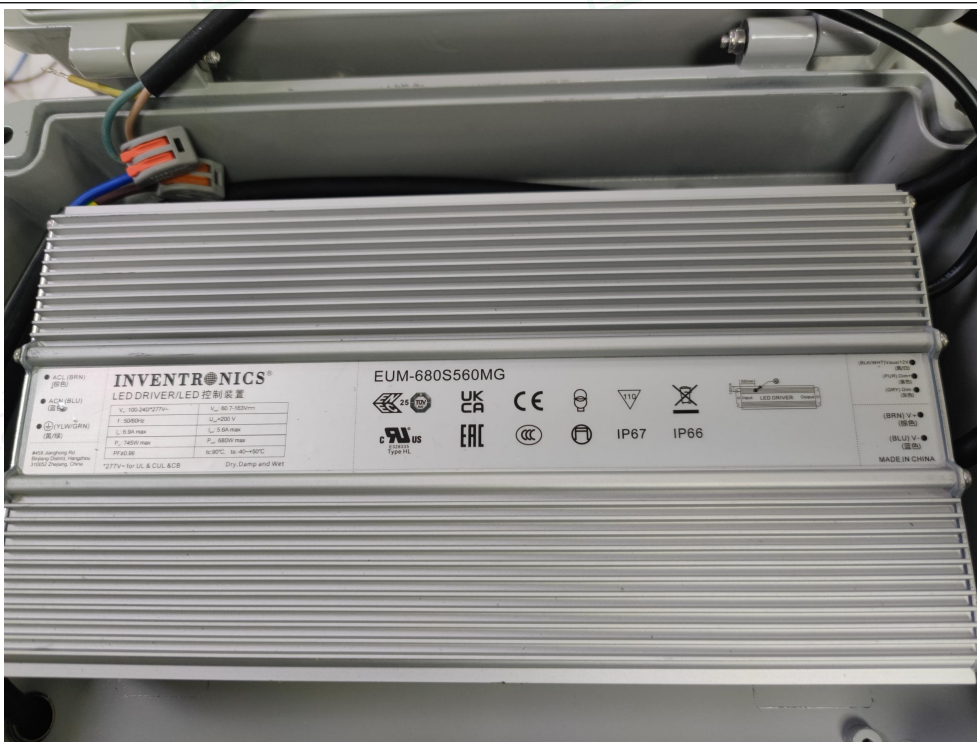
Photo 3 Label of the LED driver
