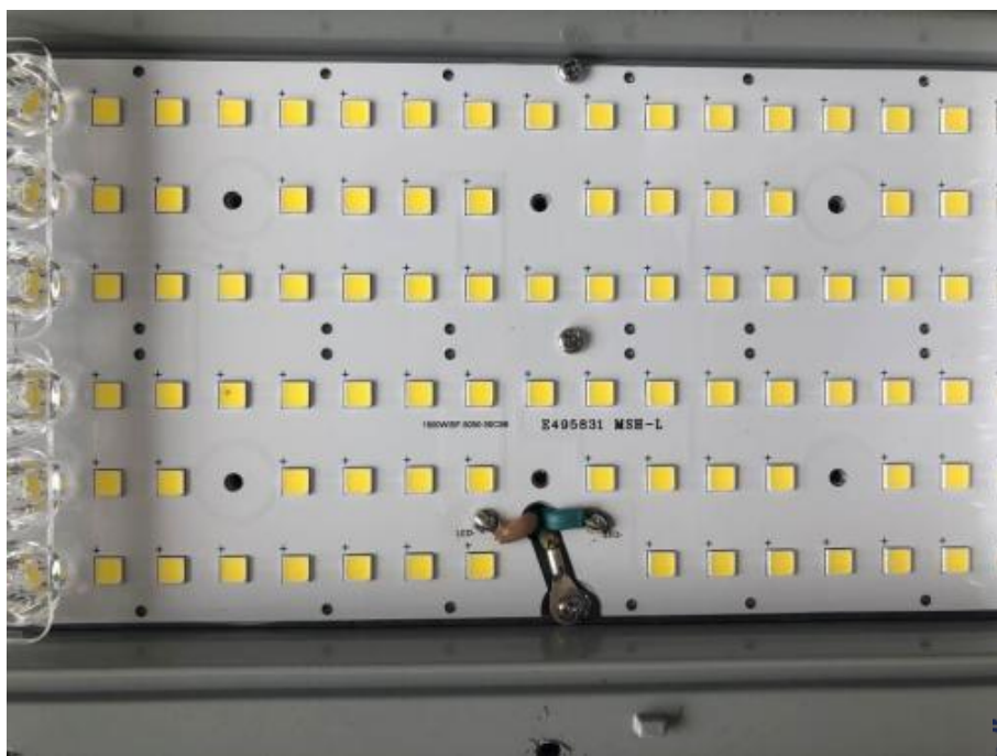
Figure 3 LED (5050) module view of model AOK-1800WiSF-HV-DV-S5-6570-30-U
