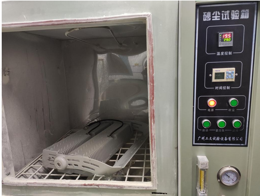
Photo 3: IP6X test of model AOK-1200WiSF-HV-00-S5-5070-30-U
