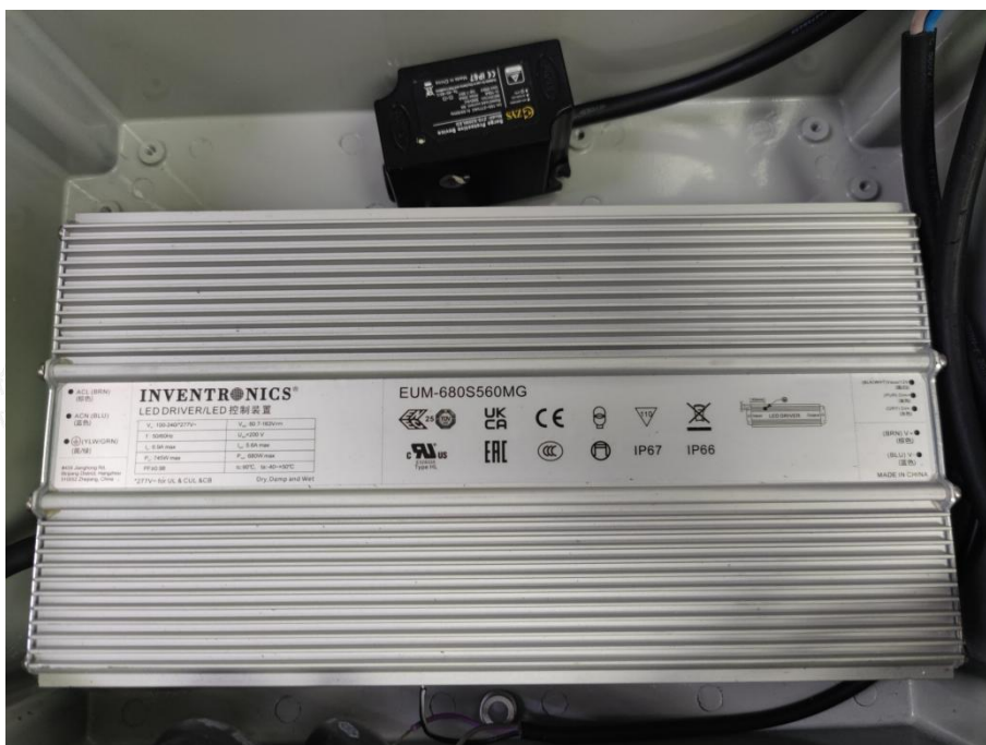
Photo 6: Test result after IP6X and IPX6 test
