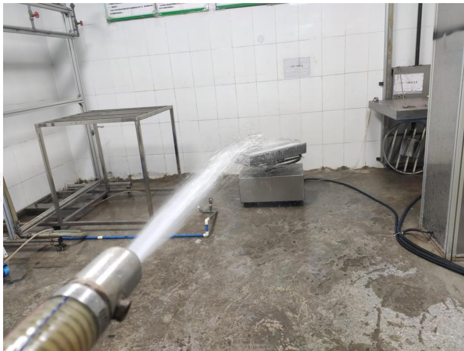
Photo 4: IPX6 test of model AOK-1200WiSF-HV-00-S5-5070-30-U
